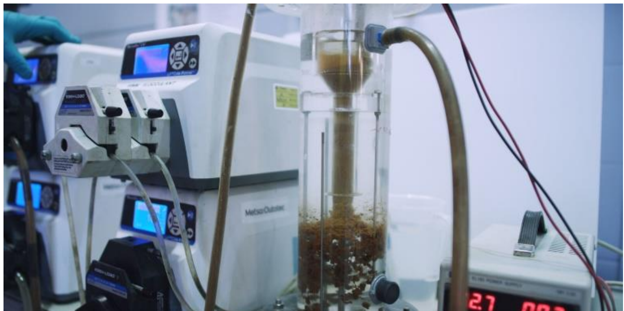
7.2 Metso's Dynamic 99 mm thickener test unit
